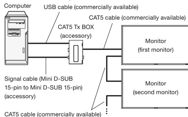
1. In addition to the connection described in 2-1), connect the OUT connector of the RGB5/CAT5 input/output connector (Modular connector 8-pin) of the first monitor and the IN connector of the RGB5/CAT5 input/output connector (Modular connector 8-pin) of the second monitor using a commercially available CAT5 cable.
