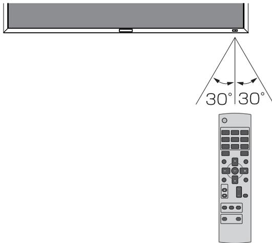
**CAUTION:** The remote control system may not function when direct sunlight or strong illumination strikes the remote control sensor of the LCD monitor, or when there is an object in the path.
