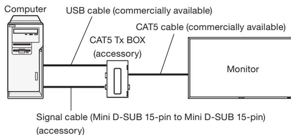
1. Connect the USB connector of the supplied CAT5 Tx BOX and that of the computer using a commercially available USB cable. (When the USB driver isn't available, connect an RS-232C cable in addition to the USB cable. In this case, the RS-232C cable serves for supplying the power to the CAT5 Tx BOX.) See page 35.
