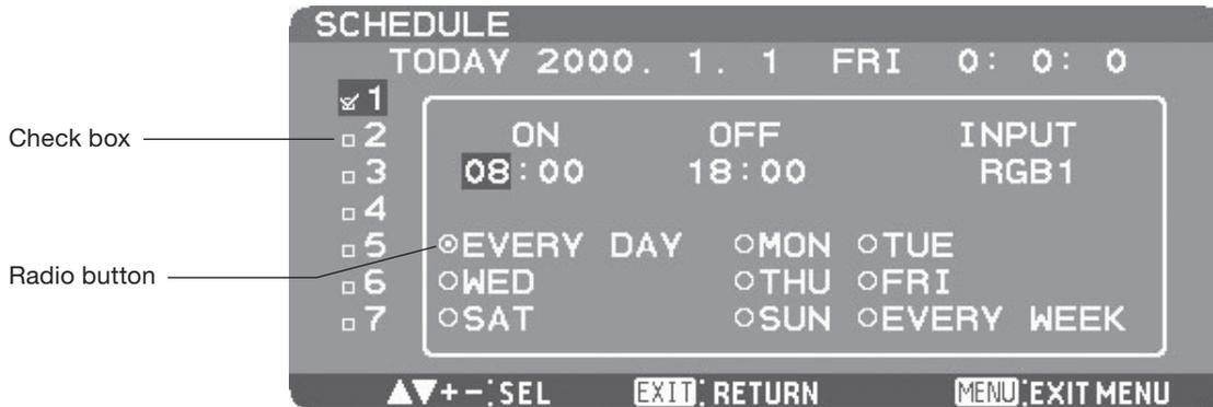
When the cursor is on any of the check boxes showing the program numbers 1 to 7 on the left side of the screen, pressing the UP (▲) or DOWN (▼) button moves the cursor vertically and pressing the PLUS (+) or MINUS (-) buttons moves it horizontally. By pressing the SET button, you can select or deselect the check boxes.
