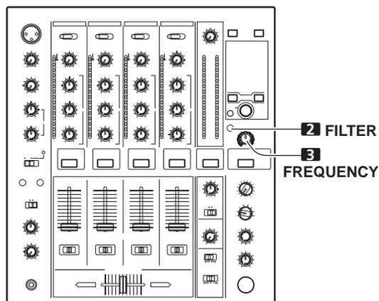
The effect frequency filter is linked to the **FREQUENCY** dial. The beat effect is applied only to the selected frequency band.
